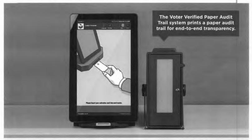
When used in the direct record electronic (DRE) configuration, the ImageCast® X can be paired with a Voter Verified Paper Audit
