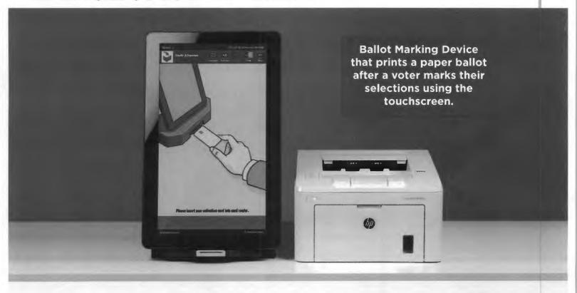
The ImageCast® X can be configured as a Ballot Marking Device (BMD), which is paired with a commercially available, compact laser printer that prints a summary of the voters selections. No votes are stored on the ImageCast® X when in the BMD configuration.
