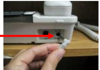
**c.** Connect the shorter telephone cord to the **EXT** socket on the back of the fax machine and to the **LINE** socket on the back of the telephone.
