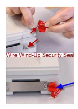
Electronic Ballot Counting Device tamper evident labels and wire wind-up seals are available through the counting device vendor.
